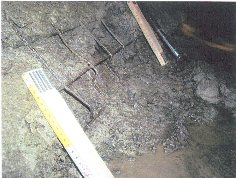
Figure 7 – Kinking of the reinforcement of the shotcrete lining due to swelling
